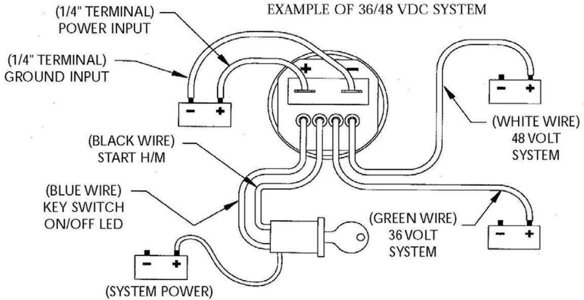
NOTE: STANDARD CABLE LENGTH IS 3 INCHES. CUSTOM CABLE LENGTH OR CONNECTOR IS OPTIONAL. ALL THE CONNECTION ARE MADE IN THE BACK OF THE METER.
